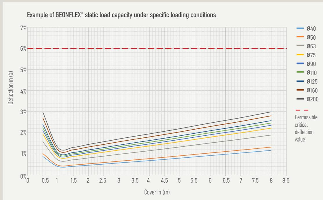
The above diagram is an example of GEONFLEX® pipes strength in specific static load under certain load conditions. It is a guide in order to be understood the degree of deflection. In NO way must be used as a specification or be confused with the specifications laid down in each individual study.
