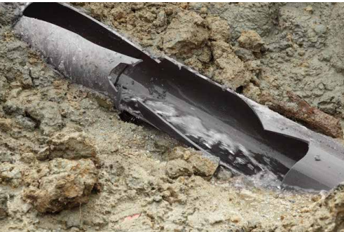
PVC pipes are more fragile and sensitive to potential knocks, due to the high levels of calcium carbonate used during their manufacturing process for cost reduction purposes.
