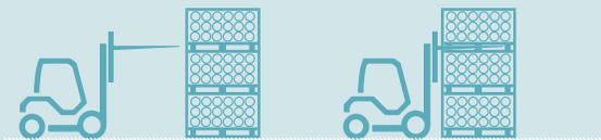
2. You can lift the pallet from its edge by placing the forks in the pallet's openings. In this case you will need larger pallet forks with minimum length 1,70m. Ensure that the forks are fully under the pallet laying under the first two wooden frames before lifting.
