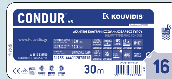
Label found on conduit bundles or coils
